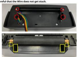
8. Reassemble the Cover DIP that was removed in step 6.
